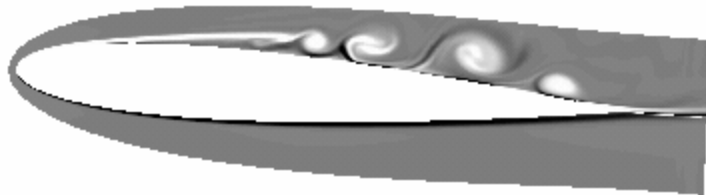
Figure 4.1.1 Contours of spanwise vorticity from 2D solution
